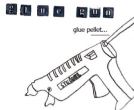
Glue guns are useful for making strong, quick joints. Use glue guns to join wood or cardboard.
