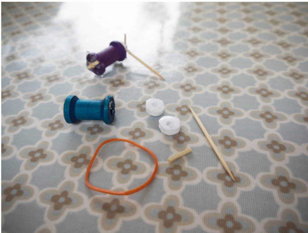
The elements of a cotton reel motor
